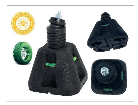
These mini adjustable feet are perfect as ground supports for AC and ASHP units. They are made from reprocessing discarded tyres where 70-95% of the rubber can be recovered. These feet are made of a blend of SBR vulcanised UV-stable rubber with internal glass fibrereinforced polypropylene.
